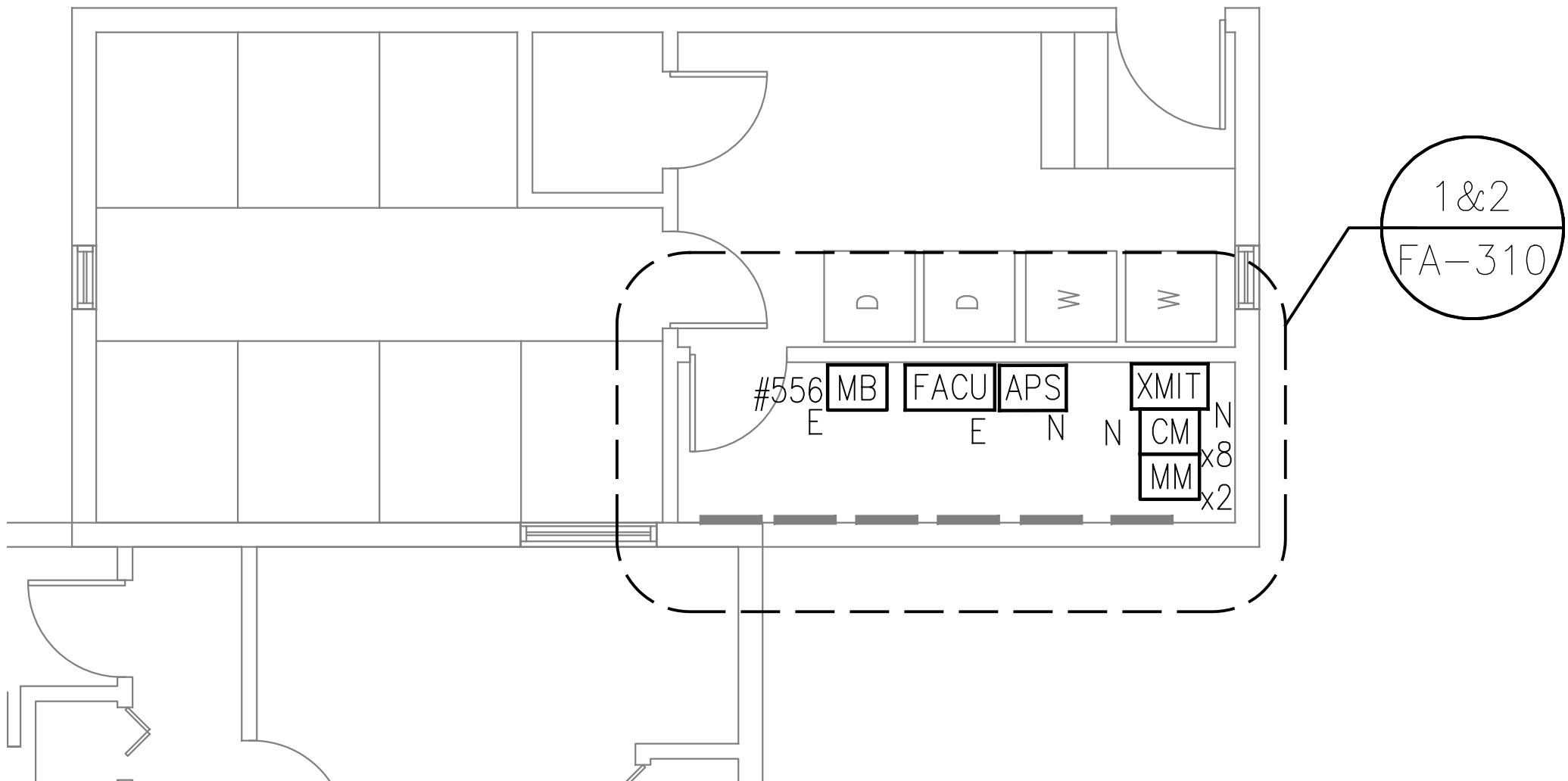
1 GRAD VILLAGE #6 - EXISTING FACP & MASTERBOX LAUNDRY ROOM - SECTION VIEW SCALE: N.T.S.
